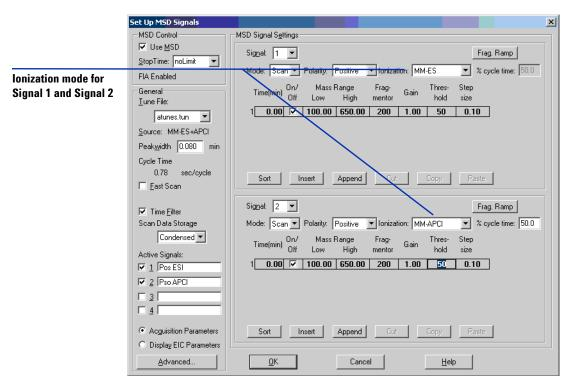
Figure 23 MM-ES and MM-APCI switching using Set Up MSD Signals dialog box
